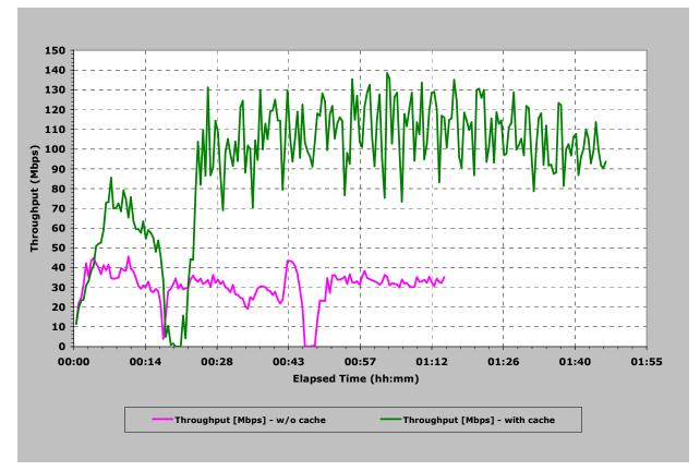
Throughput is measured in mega bits per second through the Adaptec 5445Z controller. The web server content resided on a RAID 5 partition controlled by the Adaptec 5445Z.
