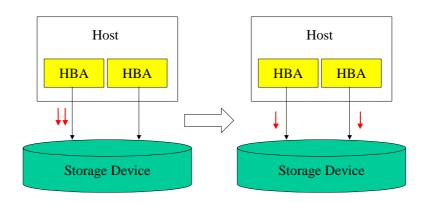
Figure 3: Load Balancing using Multipathing Devices
