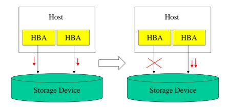
Figure 2: Fail-Over using Multipathing Devices
